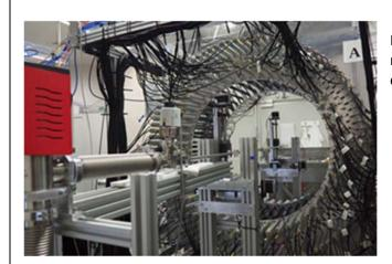
Fig. 1 J-PET detector used to perform measurements, with a small annihilation chamber inside.
