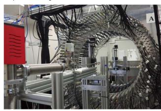
Fig. 1 J-PET detector used to perform measurements, with a small annihilation chamber inside.
